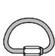
Type Q (Quick link) Connector for extra safety Quick link, "Maillon rapide"
