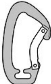
Type D (directional) Connector for Quickdraws
