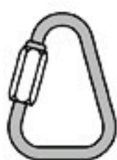
Type Q (Quick link) Connector for extra safety Quick link, "Maillon rapide"
